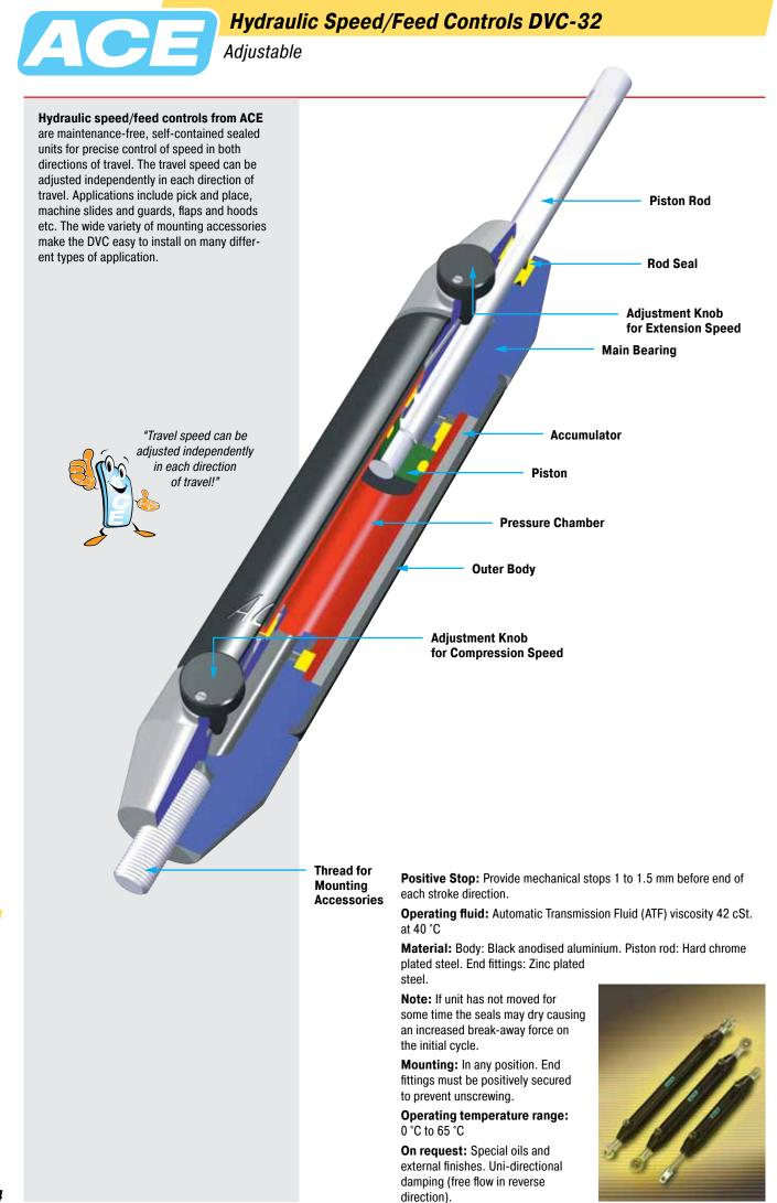
Hydraulic Speed/Feed Controls DVC-32
